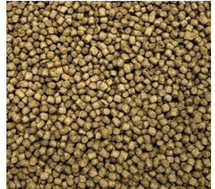
Pre-pelleting Sample Photo: 0.8mm die, 1.0mm finished product.
